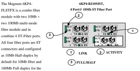
100Mb fiber. The 10Mb ST-fiber ports allow the user to connect their legacy 10Mb network to the Magnum 6K32T switch. They also provide a convenient way for the half duplex hub to connect to the switch through 10Mb fiber ports. Whereas the 100Mb ST module allow to connect the 100Mb demand of Switch devices. It supports distances according to the 10Base-FL standard i.e, 2Km distance for multi-mode fiber. (Single-mode for 10Km distance may be available as a special order).
